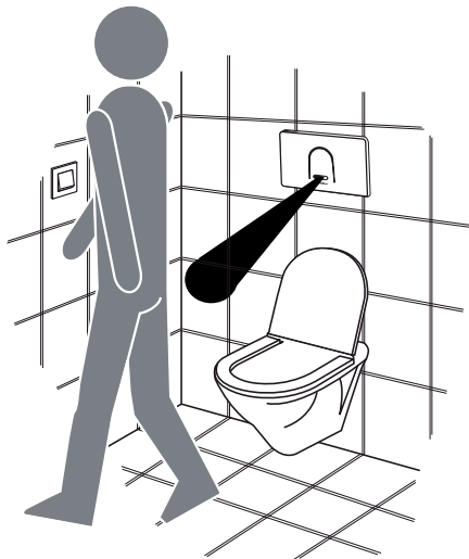
Automatic flushing after leaving the WC (switchable) Minimum stay time 15 s
