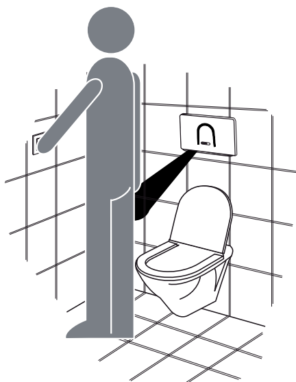
Optional intermediate flush by pressing the button
