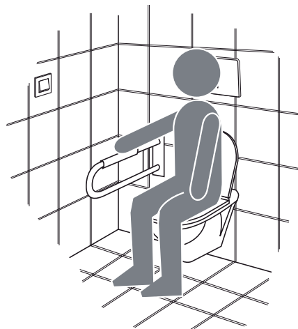
Optional intermediate flush with connection to a prop handle with integrated push button
