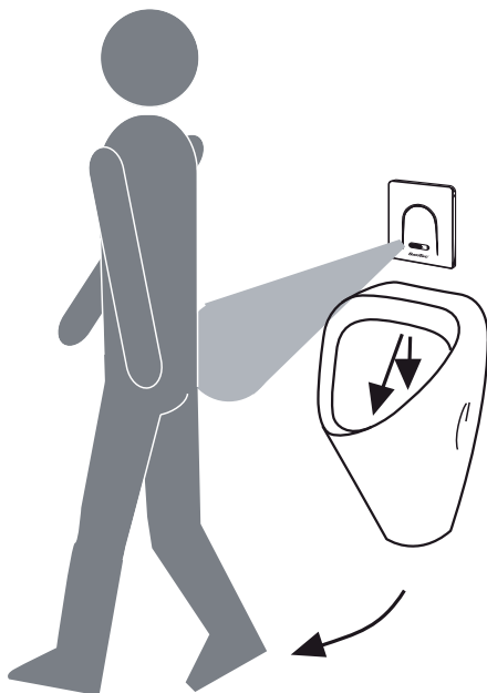
adjustable main flushing cycle from 1 to 10 secs.
