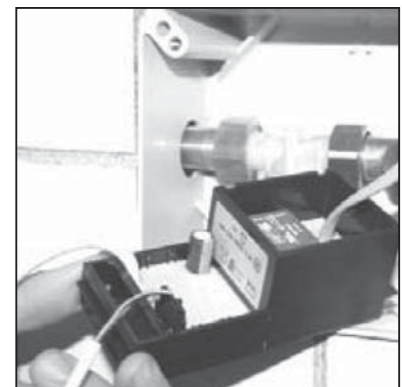
Connect sensor-siphon to electronic module
